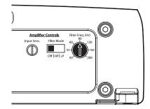
To properly set the amplifier for maximum clean output, please refer to Appendix A (page 12). After using this procedure, you can then adjust the "**Input Sens.**" level downward if this is required to achieve the desired system balance.
