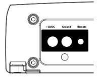
The G1300's "+12VDC" and "Ground" connections are designed to accept 8 AWG -4 AWG power wire. 8 AWG is a minimum power wire size for this amplifier.
