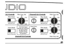
"Filter Mode" Control: The A6450 employs a 12dB per octave filter for each pair of channels (one filter for channels 1&2, another filter for channels 3&4 and a third filter for channels 5&6). Each of these filters can be configured independently into one of two filter types or defeated completely by way of the threeposition "Filter Mode" switches:
