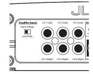
If you wish to send six discrete channels into the A6450, simply use all six inputs and set the "**Input Mode**" switch in the "**Channel 5 & 6 Controls**" section to "**Discrete**".
