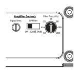
To properly set the amplifier for maximum clean output, please refer to Appendix A (page 12) in this manual. After using this procedure, you can then adjust any or all "**Input Sens**." levels downward if this is required to achieve the desired system balance.
