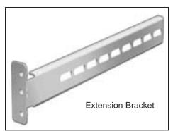
2. Affix the extension bracket to the rear of the unit using two #10-32 screws. There are 3 holes in the extension bracket for mounting. Depending on the hole pattern that is being used in the cabinet, two holes should always be available for securing the extension bracket.
