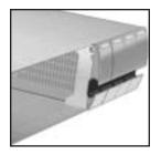
2. Pull the handle out to unlock the canister from the **FORTRA®** unit. Ensure that the thumb is placed below the line. Pressing the thumb against the Status LED lens could break it. Notice that the locking tab slides down as the handle is pulled out.
