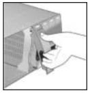
**SAFETY TIP:** After disengaging a device from the enclosure, allow 10 seconds before pulling the canister out of the unit. This allows the device to properly spin/shut down before transport.
