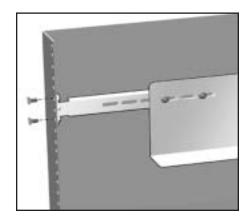
3. The fronts of the rails have three holes. Two of the holes (top and bottom) are used to secure the rail to the cabinet. The middle hole is used to secure the enclosure to the rail and cabinet. Secure the front of each rail to the cabinet vertical rails using two #10-32 screws for each rail.
