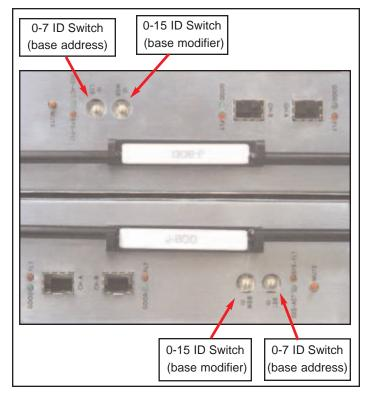
The 0-7 switch is used to set the base address which is multiplied by 16, and the 0-15 switch is used to set the offset modifier to the base address. The formula for setting the ID is: x(16)+y, where x is the 0-7 switch and y is the 0-15 switch.
