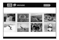
When you have selected a folder, press button for thumbnail view. Then 8 pictures are displayed on the screen. You can move through the whole folder by using the buttons: ▶ , ♠ and ▼ .
