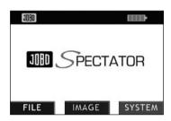
On the start up screen you can use the buttons or to select one of the three modes; FILE, IMAGE or SYSTEM mode. To confirm press the  $\ \square$  button. The selected mode is highlighted in red.
