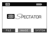
On the start up screen, you can use the buttons or to select one of the three modes; FILE, IMAGE or SYSTEM mode. To confirm press the  $\ \square$  button. The selected mode is highlighted in red.
