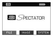
On the start up screen, you can use the buttons or to select one of the three modes; FILE, IMAGE or SYSTEM mode, To confirm press the D button. The selected mode is highlight ed in red.
