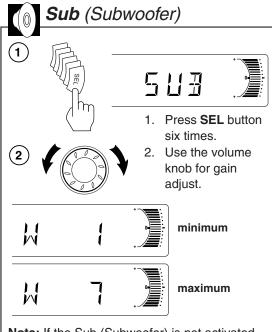
**Note:** If the Sub (Subwoofer) is not activated, the Sub (Subwoofer) function will not display.
