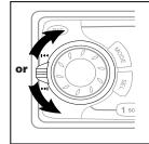
Press the Tuning Ring up or down to advance to next track. Track number appears for less than 1 second then the time remaining appears.
