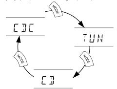
The **MODE** button only selects the CD mode if a CD is inserted, and only selects the CDC mode if a Jensen CD Changer is plugged in and a CD is inserted.
