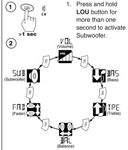
Press SEL button to move display through volume, bass, treble, balance, fader and sub functions.
