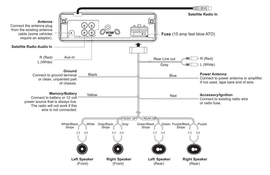
NOTE: The amplifier in this radio is only designed for use with four speakers. Never combine (bridge) outputs for use with two speakers. Never ground negative speaker leads to chassis ground. Failure to wire exactly as shown may cause electrical damage to the radio. NOTE: Only connect speakers with a nominal impedance of 4 ohms. Speakers with a load impedance less than 4 ohms could damage the unit.
