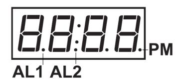
AL1: Icon lights when Alarm 1 is on. AL2: Icon lights when Alarm 2 is on.
