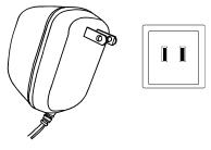
**CAUTION:** The system has an AC plug and will only fit into matching AC outlets. This is a safety feature to reduce the possibility of electric shock. If the plug will not fit in your AC outlets, you should have the outlet changed by a qualified, licensed electrician. Do not use an adaptor to make the plug fit into your outlet. This defeats the safety feature and could expose you to electric shock.
