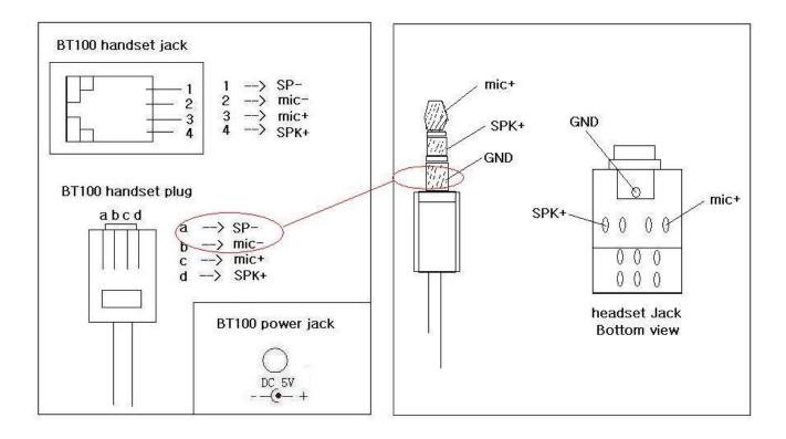
As show in the schema, the left side is pin assignment for a RJ11 interface headset; while the right side is showing a normal 3.5mm headset plug. A 3.5mm to 2.5mm plug converter is required if user want to user normal 2.5mm cell phone headset. The plug converter can be purchased from any electronics component store.
