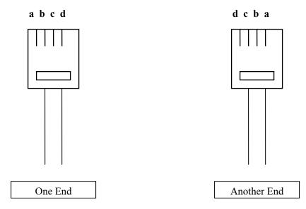
Cross Over Cable: (required to allow Plantronic Headset to work with the phone)
