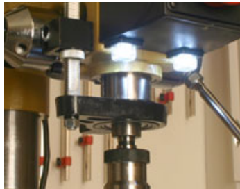
A pair of LED work lights (left) illuminate the drilling area while reducing shadows. The dual laser lights (right) are bright, easy to see and fully adjustable by the user. With the laser lines crossing exactly at the point of entry of the drill bit, hitting layout marks is fast and easy – not to mention accurate.
