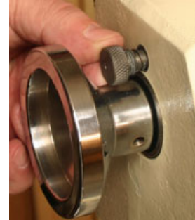
The indexing button can be held in manually for removing threaded-on accessories or it can be screwed in to free your hands for fluting or drilling operations.
