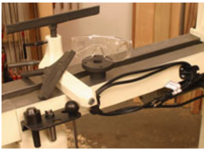
The JWL-1220VS comes with a handy tool rack and cord wrap (left) in addition to the other accessories. The handy work light (right) makes working with smaller turnings easier and safer.
