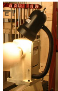
The JWL-1220VS comes with a handy tool rack and cord wrap (left) in addition to the other accessories. The handy work light (right) makes working with smaller turnings easier and safer.
