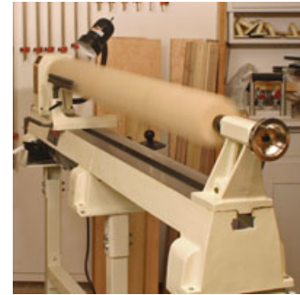
The 28" bed extension and 3/4HP motor allow turning pieces up to 50" long, a capacity rivaling far more expensive machines.
