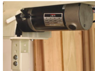
The stand features wide-stance, rubber-tipped feet (left) that adjust for irregular floors. The mounting plates (right) are adjustable up and down to fine-tune spindle height for comfort.
