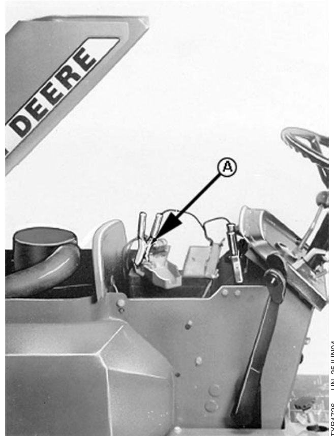
Negative Ground Connections
