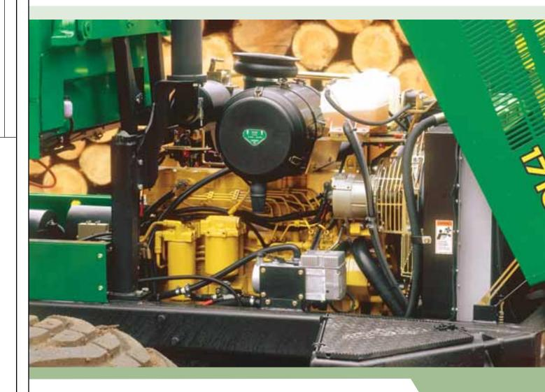
For preventative maintenance, the cab on the 1110D, 1410D and 1710D models can be hydraulically lifted and shifted to one side, and the belly pan is lowered and raised by a winch for easy access.
