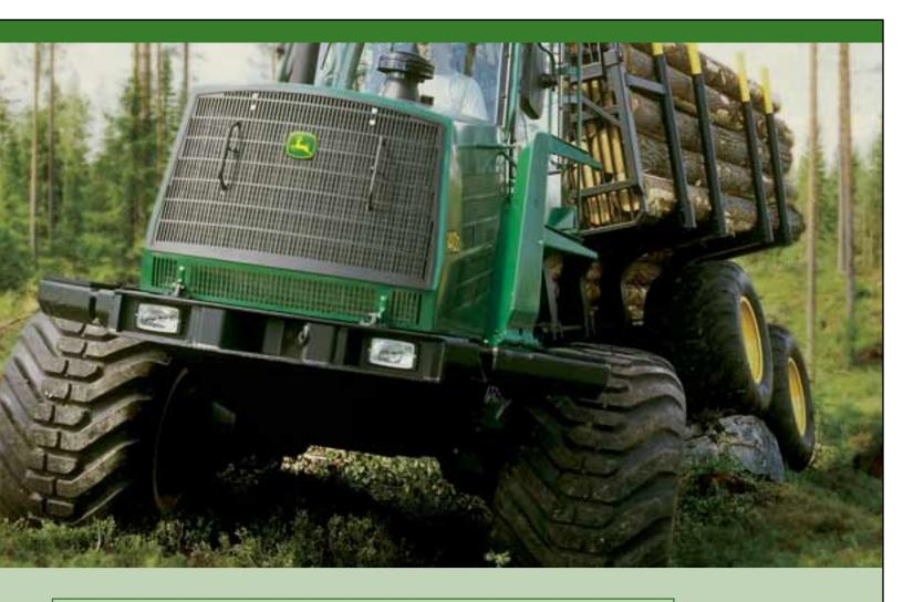
The patented balanced bogie system significantly increases the environmental friendliness of the machine. Evenly distributing the weight between all the wheels reduces the ground impact and provides a smooth ride, even when the forwarder is fully loaded.
