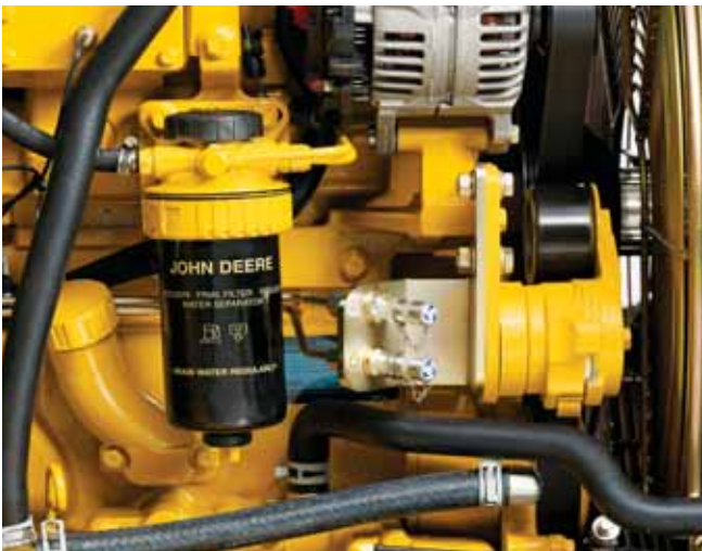
Vertical spin-on engine, transmission, and hydraulic filters and quick-release fuel filters allow quick, no-spill changes.
