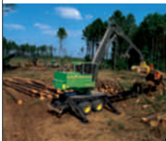
The 437C shares a common platform and engine with the 335C and 435C creating consistency across the line.
