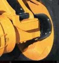
Strategically placed guards protect axle seals and help insulate the heavy-duty axles from harmful trash and contamination.
