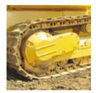
Final drives incorporate a unique oil-filled double-seal design. If a failure occurs, the oil encased between the seals escapes, setting off an indicator light on the control panel. It's an early warning system that can help prevent major final-drive failures.
