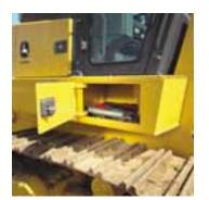
Lockable compartments on both sides of the cab provide plenty of space for storing a grease gun and tools.
