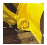
Bucket pins are oil-filled and sealed for virtually maintenance-free service and long life.
