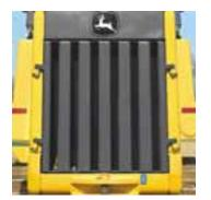
Five fin-per-inch radiator core provides efficient cooling, resists plugging, and cleans easily.
