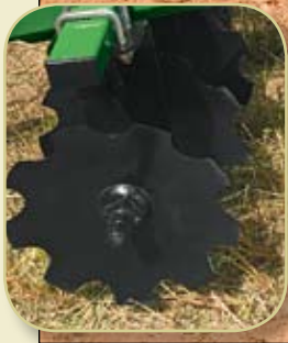
Heavy-duty notched disks turn the hardest soils into soft seed beds.
