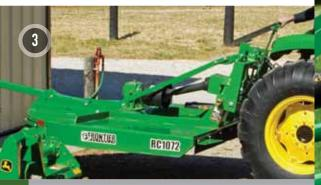
To quickly change implements with the iMatch Quick-Hitch, you simply back in, hydraulically lift the unit and secure the latches.
