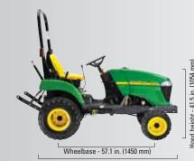
Min. width - 44.9 in. (1140 mm) Width - 47.1 in. (1196 mm)
