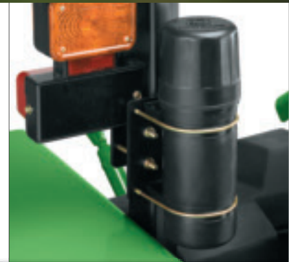
All 5003 Series Tractors come standard with storage locations for tools, parts, and operator's manuals. The toolbox is located on the left fender for easy access to tools and spare parts. The operator's manual holder is mounted on the right hand post of the ROPS for quick, easy access.
