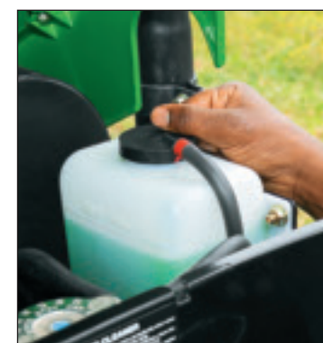
With this translucent coolant reservoir (similar to the one in your car) you can check coolant levels at a glance.
