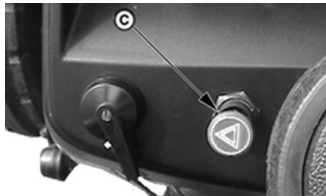
Hazard Light Switch
