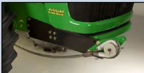
Optional steel tow cable connects to the tractor drawbar (dealer installed). It unhooks easily from the front storage pin for quick hook-ups to the tow vehicle.
