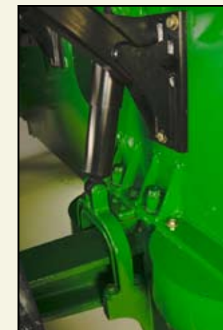
(4) Heavy-duty reaction arm (above) attaches to rear axle and pivots up and down.
