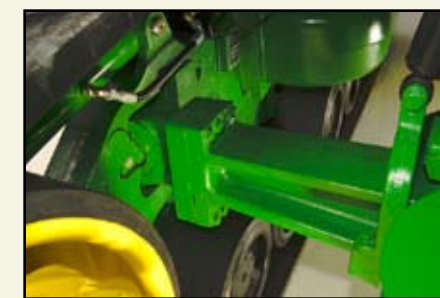
(3) Heavy-duty bushing cushions the walking beam and provides a pivot point for movement.
