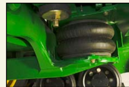
(2) Two sets of air bags in front and behind the front walking beam help cushion your ride.
