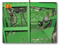
areas accessible from engine deck. Start with engine compartment and work outwards and counterclockwise to other areas around engine compartment, floor underneath engine, top rear of rotor and rear deck, including top of diesel particulate filter (if equipped). Once top areas of machine are clean, proceed to cleaning areas accessible from ground level.
