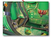
From ground level, clean rear underside of fuel tank area and top of the rear tailboard of the residue disposal system. Diesel particulate filter area (if equipped) will also need to be cleaned from ground level. Once the cleaning from ground level is finished, recheck engine compartment for any crop debris that could have blown in from ground level cleaning.
