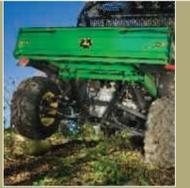
Independent rear suspension provides a full 7 inches of rear travel for a smooth ride on uneven terrain.
