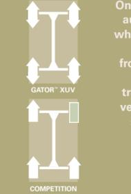
On demand, true 4WD automatically senses when rear wheels slip, then engages both front wheels with full torque, maximizing traction. Competitive vehicles with limited-slip differentials are 3-wheel drive.
