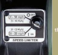
You're in control with the speed limiter kit available on the 620i. Lock in the standard 30 mph top speed or the slower 20 mph speed when needed.
