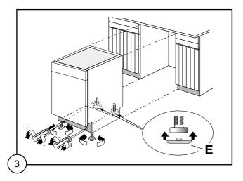
If necessary, pads (E) are supplied for the rear feet to make sliding the appliance in and out of the recess easier. To fit the pads, press them onto the rear feet. If required, the dimensions of these pads can be reduced by breaking them where marked.
