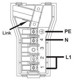
It is necessary that you install a double pole switch between the hob and the electricity supply (mains), with a minimum gap of 3 mm between the switch contacts and of a type suitable for the required load in compliance with the current rules.
