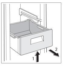
The freezing baskets have a limit stop to prevent their accidental removal or falling out. At the time of its removal from the freezer, pull the basket towards yourself and, upon reaching the end point, remove the basket by tilting its front upwards. At the time of putting it back, slightly lift the front of the basket to insert it into the freezer. Once you are over the end points, push the baskets back in their position.
