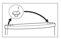
9. Unscrew the upper hinge pivot (t1) and screw it on the opposite side.
