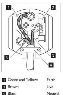
As the colours of the wires in the mains lead of this appliance may not correspond with the coloured markings identifying the terminals in your plug, proceed as follows:
