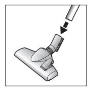
Insert the telescopic tube into the adapter of the floor tool.
