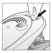
Open the lid by moving the locking lever in the direction of the arrow.
