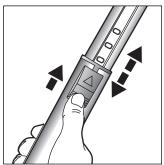
Unlock the telescopic tube to adjust its length by moving the sliding switch in the direction of the arrow.
