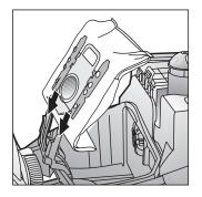
Slide the new dust bag into the holder to the stop.
