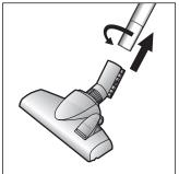
To remove it, turn the handle slightly and pull it off the tube.
