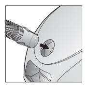
Insert the flexible hose connector into the opening on the vacuum cleaner until it engages.
