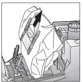
Seal the dust bag by pulling the sealing strip and then remove it.
