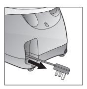
Holding the power cord by the plug, pull out the required length and plug the plug into the mains socket.
