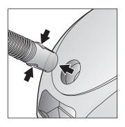
To remove the flexible tube, press the two lugs together and pull the tube out.
