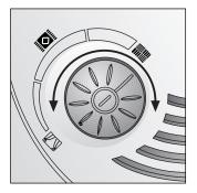
Adjust the suction by turning the on/off button in the direction of the arrow.
