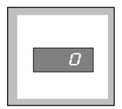
• **Delay start**, a time value indicated in hours and selected by means of the relevant button.
