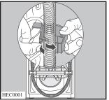
With the spanner provided unscrew and remove the central rear bolt A.
