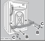
Remove the bracket **D**, refit the six smaller bolts **C** and slide out the relevant plastic spacer E.
