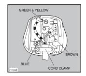
If you fit your own plug, the colours of the wires in the mains lead of your appliance may not correspond with the markings identifying the terminals in your plug.
