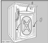
Connect the water inlet hose as described under the paragraph "Water inlet".
