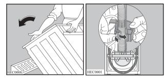
With the spanner provided unscrew and remove the central rear bolt A.
