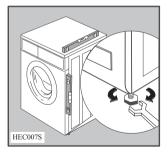
Any necessary adjustment can be made with a spanner. Accurate levelling prevents vibration, (see note on positioning), noise and displacement of the machine during operation.
