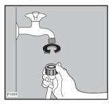
The inlet hose is provided with a water stop device, which protects against damage caused by water leaks in the hose which could develop due to natural ageing of the hose. This fault is shown by a red sector in the window "**A**". Should this occur, turn the water tap off and refer to your Service Centre to replace the hose. Installation should comply with local water authority and building regulations' requirements.
