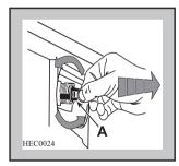
3. Remove the security gasket cup by turning and pulling it away. Pay attention not to move or remove the gasket.
