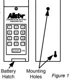
screw approximately 1/8 inch out from the wall. Slide the keypad over the screw and mark the position of the top hole. Remove the keypad and drill the top hole. Slip the keypad back over the exposed screw and finish mounting by installing the top screw. Refer to Figure 1.
