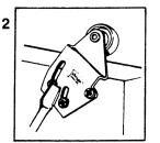
MOUNT REAR DOOR FIRST by tilting door back and resting hangers on rear rail.
