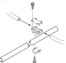
• Attach the cabling to the shaft with two cabling holders.
