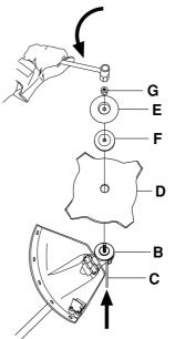
Fit the nut (G). The nut must be tightened to a torque of 35-50 Nm (3.5-5 kpm). Use the socket spanner in the tool kit. Hold the shaft of the spanner as close to the blade guard as possible. To tighten the nut, turn the spanner in the opposite direction to the direction of rotation (Caution! left-hand thread).
