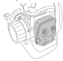
Some mufflers are equipped with a special spark arrestor mesh. If your machine has this type of muffler, you should clean the mesh at least once a week. This is best done with a wire brush.
