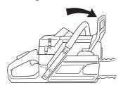
**Starting:** The chain brake should be activated when starting the chain saw. Activate the chain brake by pushing the front hand guard forwards.
