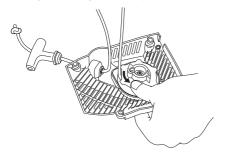
Undo the screw in the centre of the pulley and remove the pulley. Insert and fasten a new starter cord to the pulley. Wind approx. 3 turns of the starter cord onto the pulley. Connect the pulley to the recoil spring so that the end of the spring engages in the pulley. Fit the screw in the center of the pulley. Insert the starter cord through the hole in the starter housing and the starter handle. Make a secure knot in the end of the starter cord.
