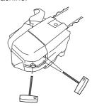
Some mufflers are equipped with a special spark arrestor mesh. If your machine has this type of muffler, you should clean the mesh at least once a week. This is best done with a wire brush. A blocked mesh will cause the engine to overheat and may lead to serious damage.
