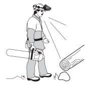
7 Take great care when cutting a tree that is in tension. A tree that is in tension may spring back to its normal position before or after being cut. If you position yourself incorrectly or make the cut in the wrong place the tree may hit you or the machine and cause you to lose control. Both situations can cause serious personal injury.
