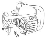
Fit the bar over the bar bolts. Place the bar in its rearmost position. Place the chain over the drive sprocket locate it in the groove on the bar. Begin on the top edge of the bar.
