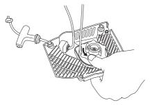
Undo the screw in the centre of the pulley and remove the pulley. Insert and fasten a new starter cord to the pulley. Wind approx. 3 turns of the starter cord onto the pulley. Connect the pulley to the recoil spring so that the end of the spring engages in the pulley. Fit the screw in the centre of the pulley. Insert the starter cord through the hole in the starter housing and the starter handle. Make a secure knot in the end of the starter cord.
