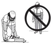
Place the chain saw on the ground and hold the rear handle down with your right foot. Grasp the front handle firmly using your left hand. Make sure the chain saw is steady and the chain is not touching the ground or other objects. Then grasp the starter handle with your right hand and pull the starter cord. Never wrap the starter cord around your hand
