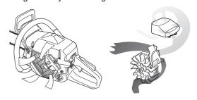
IMPORTANT! In order to maintain operation of the centrifugal cleaning system it must be regularly maintained.
