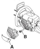
These reduce the flow of cooling air and prevent large amounts of snow from being sucked into the carburettor space. **CAUTION!** When the winter plug is fitted the winter flap must be open!
