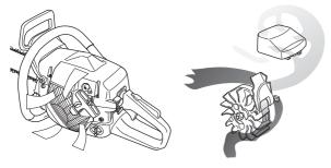
IMPORTANT! In order to maintain operation of the centrifugal cleaning system it must be regularly maintained. Clean the air intake to the starter, the fins on the flywheel, the space around the flywheel, inlet pipe and carburetor compartment.
