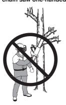
5 In order to keep control of your saw, always maintain a firm foothold. Never work on a ladder, in a tree or on any other insecure support.
