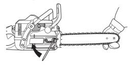
When fitting a new chain, the chain tension has to be checked frequently until the chain is run-in. Check the chain tension regularly. A correctly tensioned chain ensures good cutting performance and long life.
