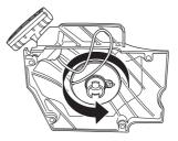
Undo the screw in the centre of the pulley and remove the pulley. Insert and fasten a new starter cord to the pulley. Wind approx. 3 turns of the starter cord onto the pulley. Connect the pulley to the recoil spring so that the end of the spring engages in the pulley. Fit the screw in the center of the pulley. Insert the starter cord through the hole in the starter housing and the starter handle. Make a secure knot in the end of the starter cord.
