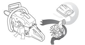
IMPORTANT! In order to maintain operation of the centrifugal cleaning system it must be regularly maintained. Clean the air intake to the starter, the fins on the flywheel, the space around the flywheel, inlet pipe and carburetor compartment.
