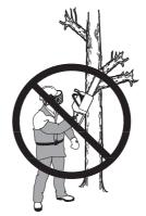
5 In order to keep control of your saw, always maintain a firm foothold. Never work on a ladder, in a tree or on any other insecure support.
