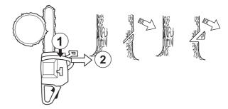
The directional cuts should run 1/4 of the diameter through the trunk and the angle between the top cut and bottom cut should be  $45^{\circ}$ .
