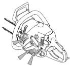
IMPORTANT! In order to maintain operation of the centrifugal cleaning system it must be regularly maintained. Clean the air intake to the starter, the fins on the flywheel, the space around the flywheel, inlet pipe and carburetor compartment.
