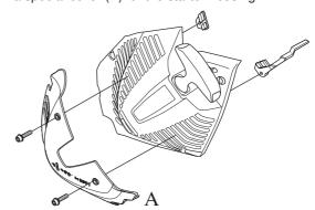
This reduces the flow of cooling air and prevents large amounts of snow from being sucked into the carburettor space.
