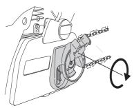
When fitting a new chain, the chain tension has to be checked frequently until the chain is run-in. Check the chain tension regularly. A correctly tensioned chain ensures good cutting performance and long life.
