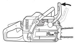
Remove the bar nuts and remove the clutch cover (chain brake). Take off the transportation ring (A).
