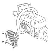
Pull out the cord approx. 30 cm (12 inches) and hook it into the notch in the rim of the pulley. Release the recoil spring by letting the pulley rotate slowly backwards.
