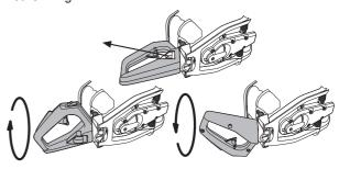
While working the handle should always be facing upwards irrespective of how the hedge trimmer is directed.
