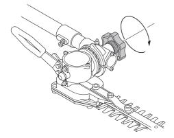
• Adjust the angle with the help of the handle on the cutting unit.
