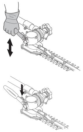
4 Fold down the cutting unit against the shaft.
