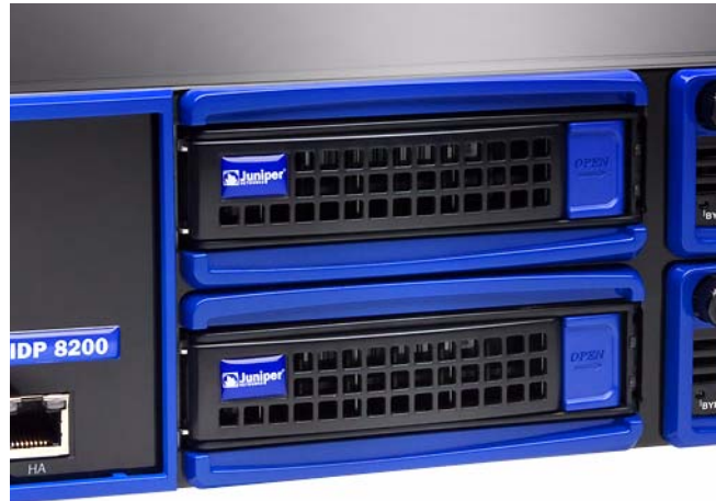
Figure 20: Hard Drive Latch in Closed Position
