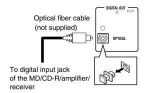
Be sure to pull off the caps before you make any connections, as shown above. Place the caps in a safe place.
