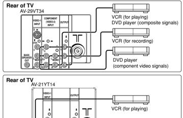
When you use VIDEO-1 INPUT, you should choose to connect S-VIDEO or video input. If S-VIDEO connector and video input are connected at the same time, no picture displays on the screen and the message "PLEASE DISCONNECT VIDEO-1 CABLE!" appears. In this case, you should disconnect either S-VIDEO or video input.
