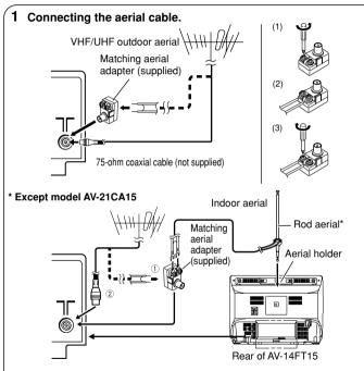
If you connect a VCR, connect the aerial output jack of your VCR and the aerial jack on the TV with the aerial cable. Then connect the output jacks of your VCR and the VIDEO-1 input jacks of the TV with the video cable and audio cables. For details, see the manual of your VCR.
